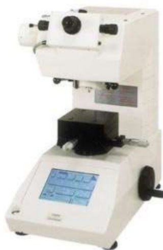
Figura 27 - Microdurômetro Shimadzu HMV-2 (UFF).
